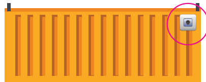
IoT device with temperature and humidity sensor mounted inside the container
